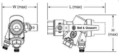
a union end with sweat, female NPT or male NPT. Valves are normally equipped with 1" long capped readout ports fitted with internal check valves.
