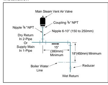
To prevent steam vents from sputtering water or damage from water hammer, observe the minimum elevations shown.
