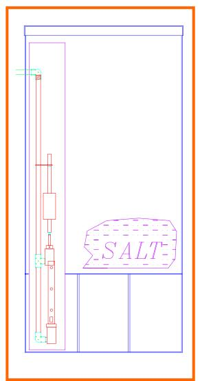
Water softeners often regenerate resin automatically. The frequency of regeneration is controlled by time or quantity of produced water. Separation of brining cycles and service flow is essential to avoid passing salt into the treated water.
