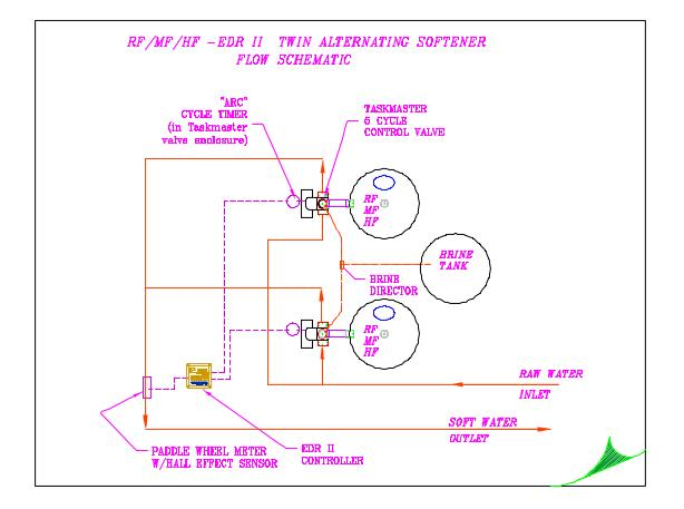
**NOTES ON DLAGRAM**. The diagram shows a configuration for a Twin Alternating system using Taskmaster valves with internal ejectors, which includes all RF and MF systems and HF systems up to HF 750.
