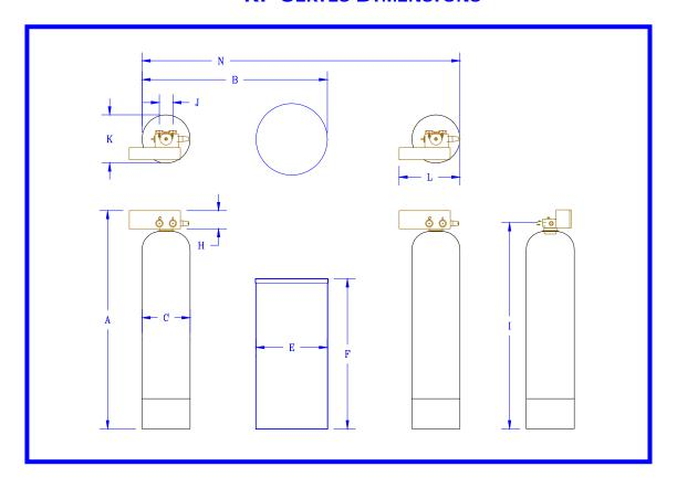
Note:  $A - Height^5$ , E - Depth, B - Single Width,  $N - Twin Width^6$ Specifications listed are not skid mounted systems. Skid dimensions given upon request.
