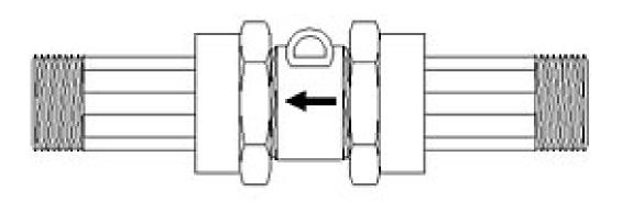
rotates, a pulse of electrical current is generated. This is called the Hall Effect. Flow is registered on an external device by counting the pulses. The paddle wheel assembly is corrosion-proof Noryl®, with a ceramic-encased magnet and stainless steel shaft.
