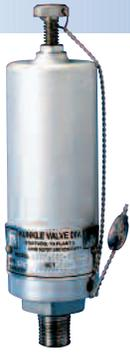
**Models 230, 330, 330S and 333S** Lightweight aluminum construction, resistant to environmental and internal corrosion. Opening pressure is repetitively consistent, relief action is smooth, reseating is positive with minimum pressure drop. The full spring load is never imparted to synthetic disc insert. Seat tightness increases to a maximum as inlet pressure approaches the opening pressure.
