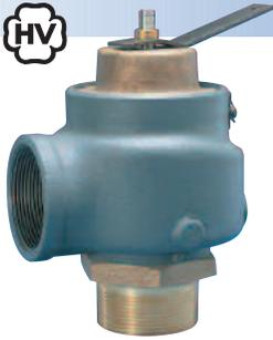
**Model 930** Extra high capacity for industrial, commercial and residential low pressure steam heating boilers. Cast iron with bronze nozzle, disc and guide. Large seat area/guide area ratio, along with disc pivot design insures top valve performance. Flat bronze valve seats are lapped for optimum performance. Reversible lift lever for 'pull-up' or 'pull-down' manual testing.
