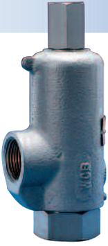
**Models 71S and 171** Extra heavy, rugged construction. Seats lapped for optimum performance. Ball bearing pivot between disc and spring corrects misalignment and compensates for spring side thrust.
