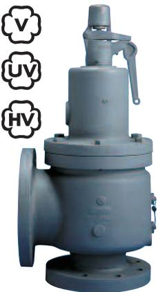
**Models 6252 and 6254** Heavy duty construction of high quality cast iron with stainless steel semi-nozzle trim. Bolted bonnet design for easy maintenance. Seats lapped to optical flatness. Dual control rings offer easy adjustability for precision opening with minimum pre-open or simmer and exact blowdown control. Heavy duty lift lever assembly.
