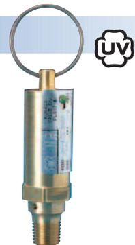
**Models 40R and 40RL** All parts are stainless steel. Precision lapped beveled seats for optimum performance. Pivot between spring and disc corrects misalignment and compensates for spring side thrust.
