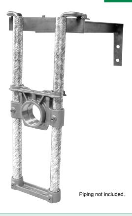
Rail systems are used for easy pump removal from an effluent pit. Service personnel will not need to enter a hazardous environment. Pump sits on floor and engages piping system via a sliding disconnect fitting. All parts are stainless steel or brass and suitable for a septic environment.
