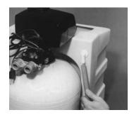
22. Install 1/2" I.D. rigid or non-collapsible tubing (not included) to the overflow hose barb located on the back of the softener brine tank and run to a drain located below the level of the hose barb.
