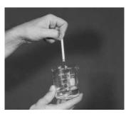
3. Draw untreated water sample into container. Open test kit and dip tester into water sample.
