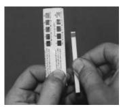
4. Compare strip with chart to determine water hardness. Retain this number for setting control valve later in the installation process.
