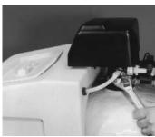
Loosen compression nut located on right side of control valve by turning counter clockwise. Insert end of 3/8" O.D. tube, making sure tube is pushed in fully. Visually check brine tubing for cracks or kinks. Tighten the compression nut.
