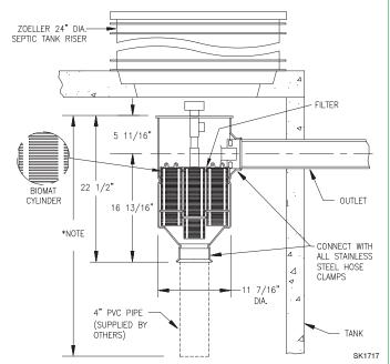
\*NOTE: State and local plumbing codes may require a specific liquid penetration. For example, 25% - 45% into the liquid depth or 9" off the tank bottom.
