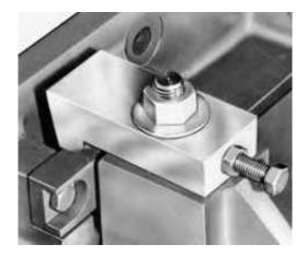
The side wedge system, used on all gates, is the most critical. It must resist the vertical loads placed on the gate when closing and assumes most of the unseating head loads. Because it is virtually impossible to spread these forces equally on all wedges, the loads assumed by the side wedge system can be high.
