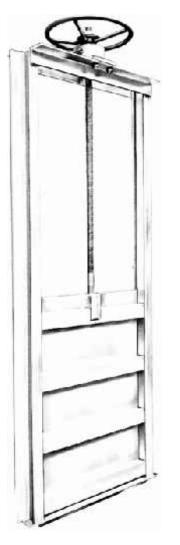
connection, welded, not only to the disc, but to the top reinforcing rib as well. This gate is normally supplied with a resilient seal attached to the bottom of the disc for flush-bottom closure. The design of the guides and yoke allows removal of disc and stem without disassembling the yoke.
