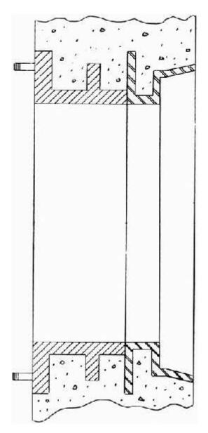
is used, the two flanges can be bolted or clamped together. If the concrete pipe manufacturer can furnish a spigot suitable for a cast iron pipe bell, Rodney Hunt can furnish a flange and bell wall thimble.
