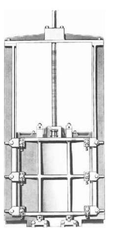
What is a self-contained sluice gate? The self-contained gate differs from the conventional gate in that it absorbs the operating load created during opening and closing. This is accomplished through the use of a yoke or supporting member mounted on the top of extended guides. The force required to operate the gate is transmitted by the yoke and guides directly back to the gate.
