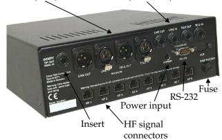
RS-232 serial port for remote control applications such as *Close Talk Control* PC software for conference control and *Close Talk Install* PC software for system testing.
