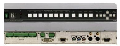
The VP-723xl is an 7-input scaler/switcher with unbalanced stereo audio. It scales any composite, s-Video (Y/C), component video (YUV), DVI video or computer graphics video signal up or down to a selectable graphics or HDTV output resolution and provides glitch-free switching between sources through FTB<sup>TM</sup> (fadthru-black) switching technology.
