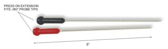
This 5" extended tip presses onto any standard probe tip with .080" Dia. tip, and allows the user to reach difficult areas, it also has a stainless steel tip with a polished point for insulation piercing or penetrating coated connections. The tip is fully insulated to the point to prevent shorting.
