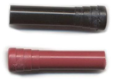
This insulator accepts Oldaker P/N 456C Jack and when pressed together becomes a shrouded 4MM safety jack. Material:: ABS V0/94 Flame retardant Plastic. Total length 1.5", Colors available, Red, Black, Blue, Green, Yellow, White. **Sold** 2 of one color per package. Bulk pricing available.
