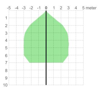
Operating range is equipment dependent. The figure above shows a radiation diagram together with the DU-111-02 Delegate Unit where the horizontal axis shows radiation diameter at ceiling heights up to seven metres.
