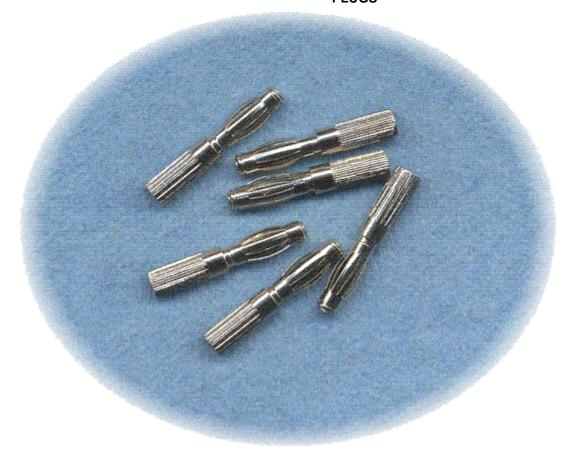
This plug base is made of 3/16" brass, Nickel Plated, and uses a 9 leaf spring contact and fits 4MM Jack. Solder Connection. Total length 1". Plug length 9/16"
