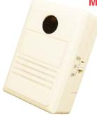
Learn the basics of motion detector technology while building this motion detector kit that uses an infrared sensor. Use as a burglar alarm, message minder, room detector, or entry to home or business.
