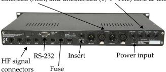
RS-232 serial port for remote control applications such as *Close Talk Control* PC software for conference control and *Close Talk Install* PC software for system testing.
