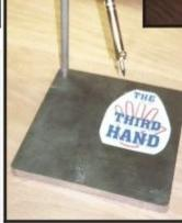
This handy fixture gives the user a 3rd hand, it holds the iron in place while you assemble and solder. 2 way adjustment with replacement parts available. Made of aluminum and measures  $6" \times 6' \times 12"$
