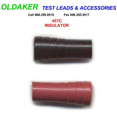
This insulator accepts Oldaker P/N's 450, 491 and 284-3 Pins & Plugs, and when pressed together becomes a unshrouded plug assembly. Material:: ABS V0/94 Flame retardant Plastic. Total length 1", Colors available, Red, Black, Blue, Green, Yellow, White. **Sold** 2 of one color per package. Bulk pricing available.
