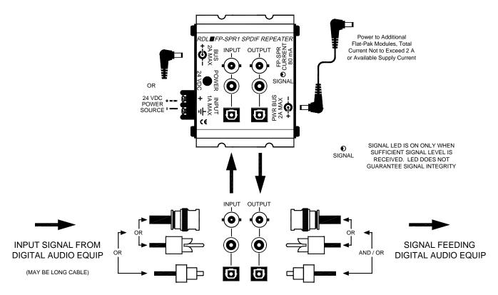
NOTE: IF FP-SPR1 IS BEING USED TO RECOVER CORRECT SIGNALS FROM A LONG CABLE, INSTALL FP-SPR1 AT THE RECEIVING END OF THE CABLE
