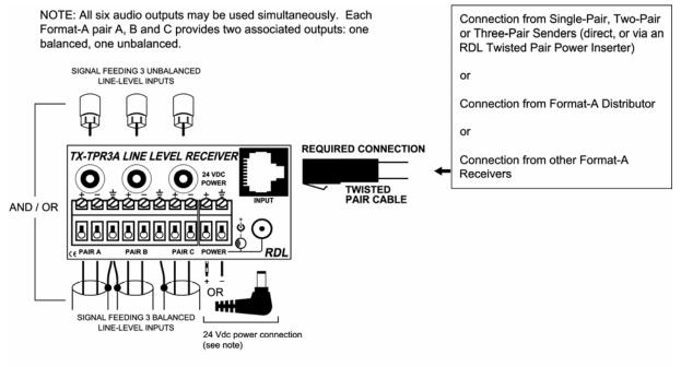
NOTE: Connect a 24 Vdc power supply to the module if power is not being supplied through a twisted pair cable from a connected module.
