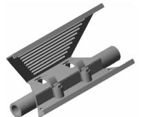
Install mounting bracket to flat surface using either the screw holes or slots provided for the mounting screws.
