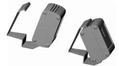
Secure the unit in the mounting bracket: •First, seat the bottom bracket in the SAS-HC8 bottom rear slot; •Then tilt the unit back until it snaps and locks into position.
