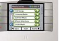
The optional UNO-TS2 keypad, when used with the SMS3 Media Server and RNET controller allows the user to make music requests
