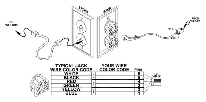
Prior to attaching jacks to all the installed wiring, we recommend verifying wire polarization by installing jacks to one set of wiring and observing proper operation of a single SAS-SM8.
