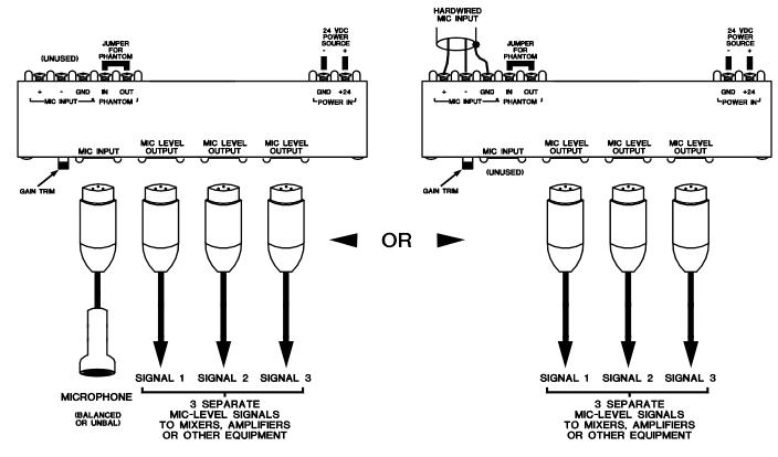
**AUDIO INPUT**: The + and - balanced audio signal enters the unit through the front-panel XLR connector, or through the rearpanel barrier strip. Inputs are normally set up for dynamic mics (no phantom). If phantom power is desired, simply jumper the **PHANTOM** terminals on the barrier strip. Unbalanced audio may be connected to the + terminal, with the unbalanced shield connected to both the - and **GND** terminal (Pin 1).
