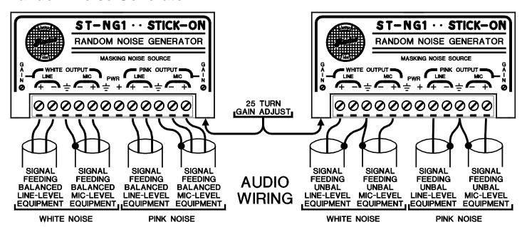
EACH OUTPUT MAY BE WIRED BALANCED OR UNBALANCED
