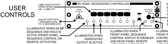
SEQUENCE CONTROL SWITCH IN THE DEPRESSED POSITION CAUSES OUTPUTS TO SEQUENCE UP; RELEASING THE SWITCH CAUSES OUTPUTS TO SEQUENCE DOWN.
