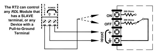
Functional Equivalent to Internal Solid State Switching Circuit
