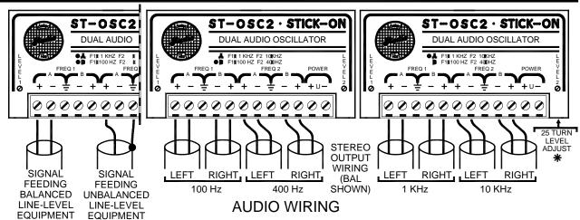
\* NOTE: THE 'LEVEL' POTS CONTROL "A" AND "B" OUTPUTS TOGETHER
