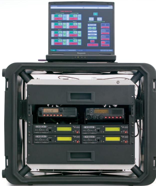
The idea behind V.I.P.E.R. is a fairly simple one. By using our innovative VoIP technology, the radio's transmissions and control information are converted into digital data—regardless of frequency or standard, VHF, UHF or 800MHz.
