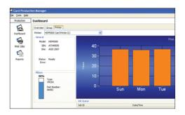
View real-time feedback on the system load to the OnQueue server as well as the number of cards printed per hour and per day by site, printer group or individual printer.
