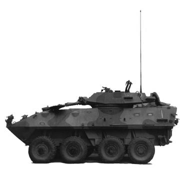
The Telex 4331 and 4332 (AS-3885) are broad-band VHF vehicular antennas covering the 30-88 MHz tactical FM frequency band. The model 4334 covers the extended frequency range of 30-108 MHz. The center fed design minimizes variations in gain and radiation characteristics when isolated from a ground plane. The mounting configuration of these antennas is identical to those of other vehicular antennas such as the AS-1729 and AS-3900.
