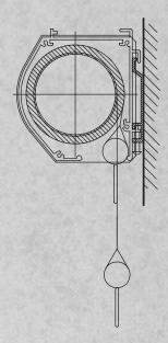
The HD II and HD III deluxe manual wall screens are designed for both home theatre and commercial applications. The HD II with a 2" roller is available in 4:3 video format in sizes from 60" to 84" diagonal. The HD III comes with 3" heavy duty roller in 4:3 video format in sizes from 100" to 180" diagonal and in 16:9 format in sizes from 92" to 147" diagonal.
