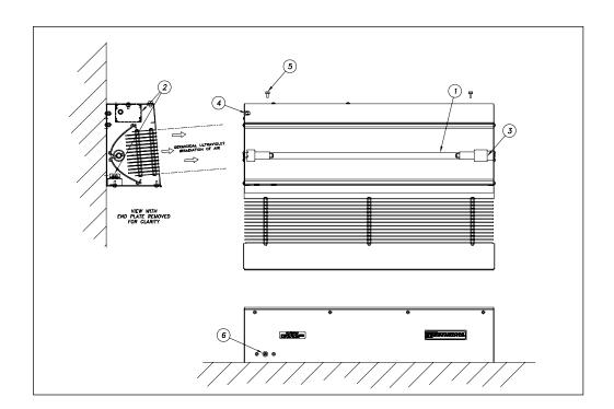
Figure 3 - Replacement parts Model LIND 24-EVO
