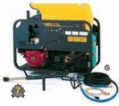
The MHP is an economy mini-skid, hot-water pressure washer with an extra narrow frame for maneuvering through doorways. Less than 25-inches in width, the MHP models is also powered by electric-start Honda or Vanguard engines. The narrow-frame chassis is made of rugged 11/4-inch steel and the Schedule 80 heating coil is backed by a 5-year warranty and protected by an aluminized steel inner wrap. The MHP also utilizes a 12V burner assembly for heating water (battery not included).
