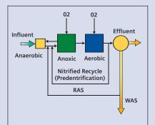
Aerated Anoxic with Anaerobic Selector Nitrogen and Phosphorus Removal
