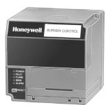
Microprocessor-based integrated burner control for industrial process semi-automatically fired gas, oil, coal, or combination fuels for single and multiple burner applications. Provides level of safety, functional capability and features beyond conventional controls.
