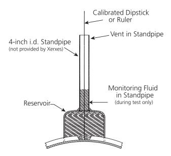
To conduct a TRUCHEK test, follow the TRUCHEK Tank-Tightness Testing Procedure outlined in this brochure and fill in the attached TRUCHEK Data Log form as appropriate for the diameter size of the tank to be tested. Keep the completed form as part of the tank records that may be required by federal, state and/or local regulations or codes.
