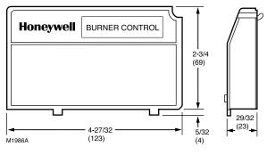
Ambient Temperature Rating: -40 F to 140 F (-40 C to 60 C)
