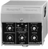
Line voltage pressure controller that provides automatic operating control, automatic limit protection, manual reset limit protection, or modulating firing rate control for pressure systems up to 300 psi.
