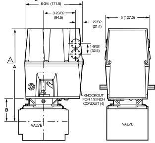
ALLOW 4 IN. (101.6 MM) CLEARANCE FOR ACTUATOR REMOVAL.
