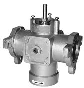
The V5197A is a firing rate valve used to provide variable flow control of air, natural gas, liquefied petroleum (LP), and manufactured gases. The V5197A is actuated by a firing rate motor that can be mounted directly on the valve. The V5197A is not applicable as a safety shutoff valve.
