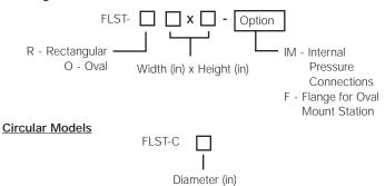
**Note:** When ordering rectangular or oval flow stations, pressure taps will always be located on the longer of the two dimensions.
