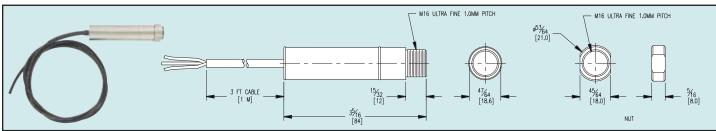
The Series ILA Non-Contact Sensors, measure temperatures from 32 to 932°F (0 to 500°C) and provide a linear 4 to 20 mA, 0 to 5 VDC or thermocouple output. The 2-wire signal is compatible with almost any indicator, controller, recorder, data logger, etc., without the need for special interfacing or signal conditioning. They are suitable for most materials such as food, paper, textiles, plastics, leather, tobacco, pharmaceuticals, chemicals, rubber, coal, and asphalt.
