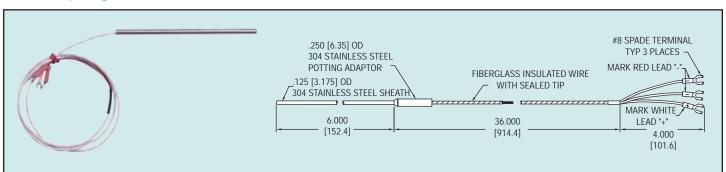
Precision RTD (Resistance Temperature Detector) offers excellent accuracy and stability over a wide temperature range. Industry standard 3-wire 100 ohm (DIN) probes are available in 6" (15 cm), 12" (30.5 cm), or 18" (46 cm) sheath lengths with 30" (76 cm) extension cable and spade lug terminals.
