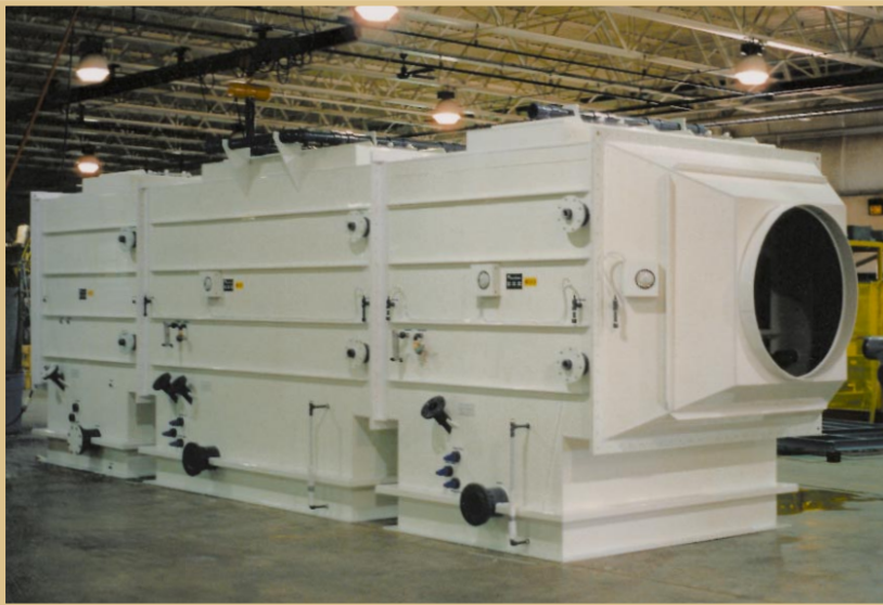
Material of Construction: 100% Corrosion Resistant UV Stabilized PVC (3/8" to 1/2" thick) Application: Wastewater Treatment Plant Odors Problem: H 2 S, NH 3 Solution: Multi-Stage, Multi-Chemistry Horizontal Cross Flow F Series Scrubber
