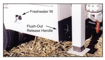
The conveniently mounted fresh water rinse tank is shown on the left, and the Stellar exclusive calcium chloride Flush-Out release handle on the right.
