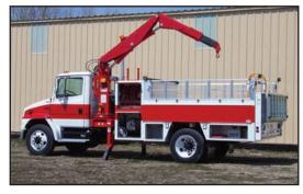
optional wheel well lights. The body of the 1184-14 AG features a drop-down floor to give a low center of gravity for the 400 gal. calcium chloride tank. This allows for maximum storage of the tank, maximum hauling space for the tires, and eliminates any interference with the crane.
