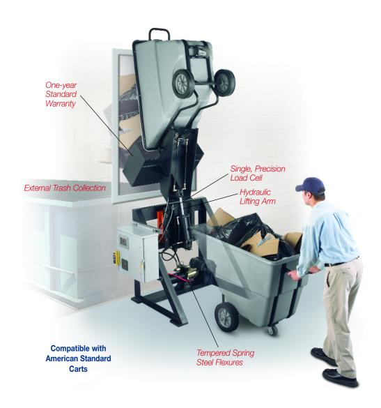
The "Smart Dumper System" combines a legal-for-trade weighing system and an easy-to-operate, hydraulic cart dumping unit. It incorporates the accuracy and durability of the LTS scale with the quality and reliability of an Ameri-Kart dumping system.
