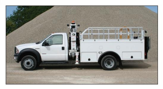
The Stellar Aggressor 1100 AR (aluminum rack) is an 11' all aluminum body built with Stellar's exclusive plank flooring. The aluminum extruded plank flooring gives the 1100 AR body unmatched strength and durability while reducing weight, thus more payload.
